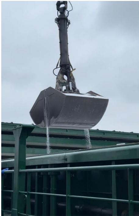
Example photos of leaking grab buckets in Polish port terminals
