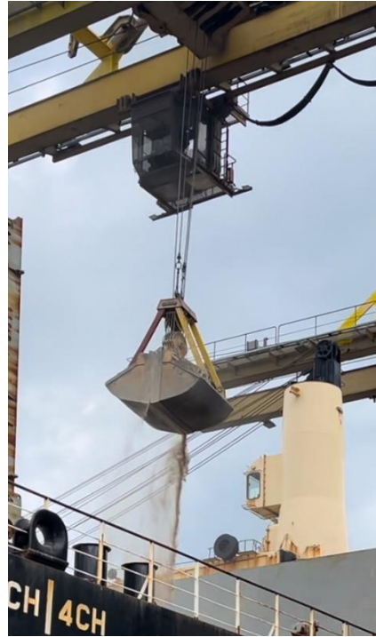
Example photos of leaking grab buckets in Polish port terminals
