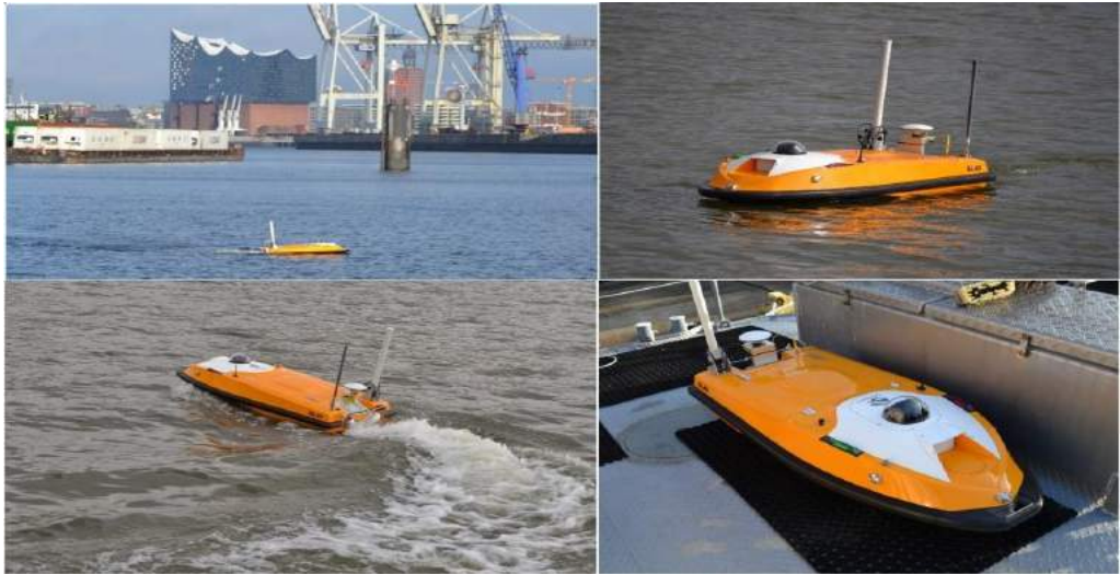
Figure 1.4. SL40 USV in port of Hamburg (Ocean Alpha 2023d, p. 104; Galdorisi 2023) (the tests of using USV for safety monitoring purposes in the port waters were conducted in 2022 at the Port of Los Angeles)
