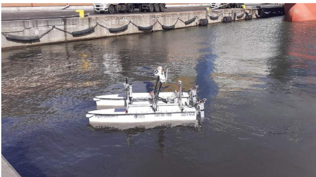
Figure 2.6. The HydroDron-1 unmanned water platform during measurements at the Rotterdam Quay in the Gdynia seaport, conducted in May 2023 year (A. Stateczny)
