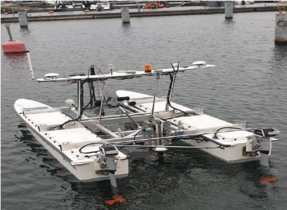
Figure 2.5. Unmanned surface vessel HydroDron-1 – view from the stern with electric motors (A. Stateczny)
