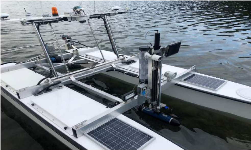
Figure 2.4. The unmanned surface platform HydroDron-1 with the multibeam sonar head in the upper position and the sound sensor mounted above the head – a view from the front at an angle (A. Stateczny)
