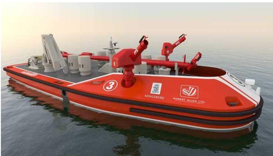
Figure 1.2. Remote-Controlled Fire-Fighting Boat (KONGSBERG, 2023)
