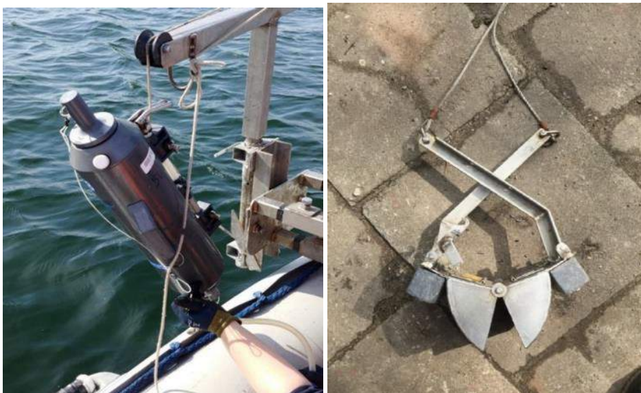
Figure 3.3. The equipment used for sampling marine waters in the basins of the Port of Gdynia includes a bathometer (on the left), while for sampling marine sediments, a Van Veen grab sampler is used (on the right) (B. Lednicka)
